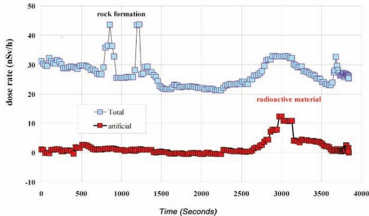
The graph above depicts two simultaneous signals, both from an identical gamma-sensitive detector. The upper (blue) line represents the normal "gross" count channel as produced from a normal system using standard counting technologies. The lower (red) signal is generated by the NBR technology driven channel which ignores natural background influences.
