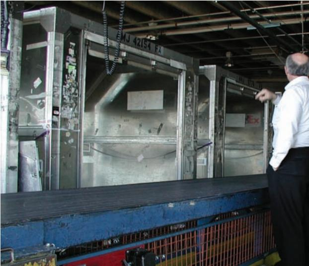
SGSII-6000GN2, four 1500 detectors for increased vertical height coverage
